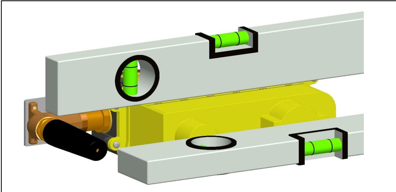
**Secure the box to the wall by using screws and bosses (not supplied) according to the type of support (wood, concrete, etc.)**
